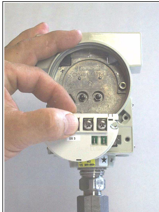
Figure 26 Pulled-out connection board with the feed-thru pins behind it
