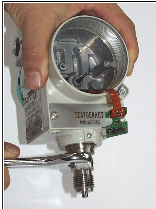
Figure 29 Loosening the cell with a fork wrench
