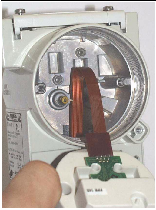
Figure 34 Looping the conductor band
