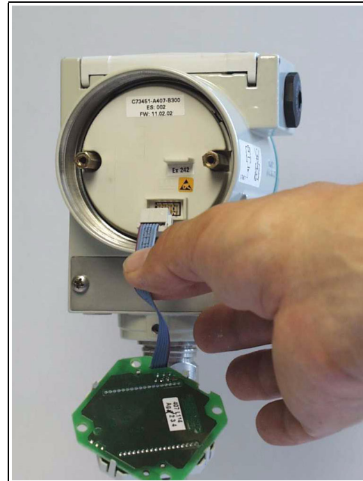
Figure 7 Pull off the LCD display until product release 29
