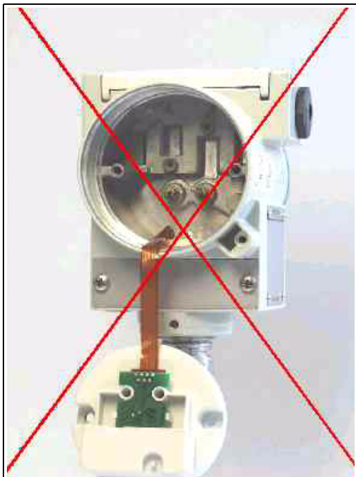
Figure 12 The conductor band should not be stretched
