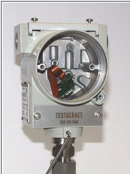
Figure 28 Loosening the locking screw with an allen wrench
