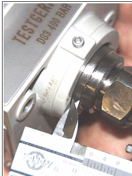
Figure 33 Observing the distance of 2.6 \text{ mm} \pm 0,75
