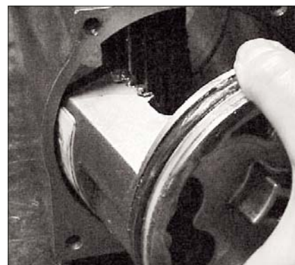
2. Fitting pistons into body
