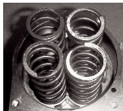
3. Locating of springs in piston head cavities
