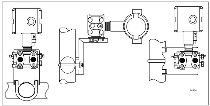
Figure 3—Examples of typical mounting positions
