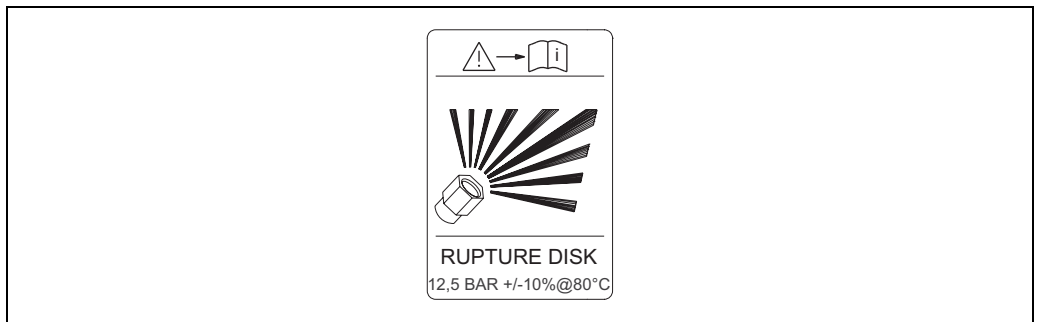
Indication label for the rupture disk
