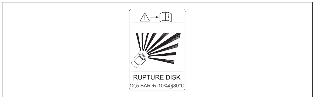
Indication label for the rupture disk
