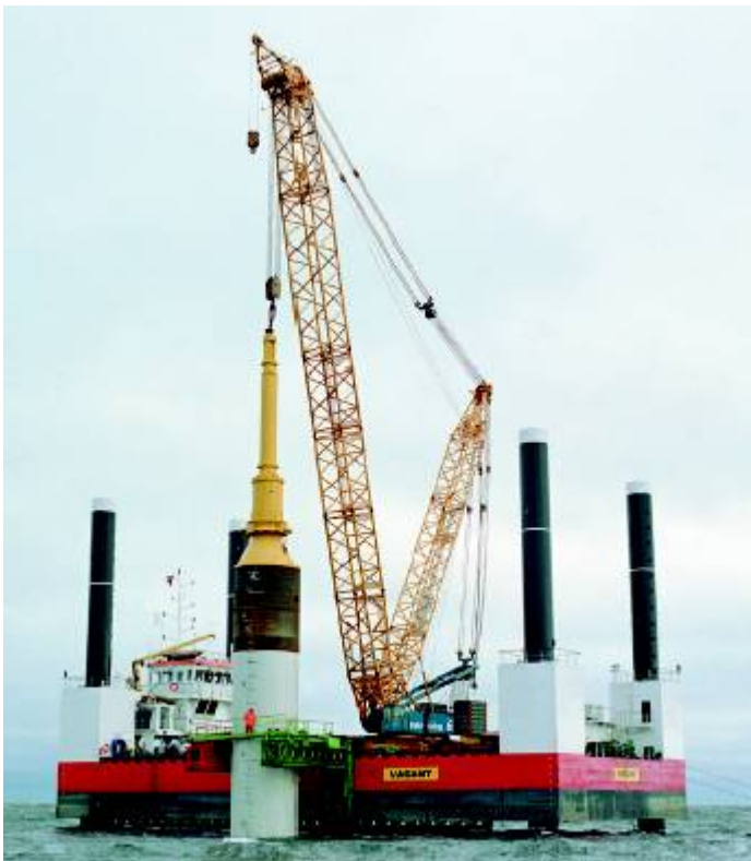
Figure 3-4: Vagant Jack-up platform used for soil investigations.
