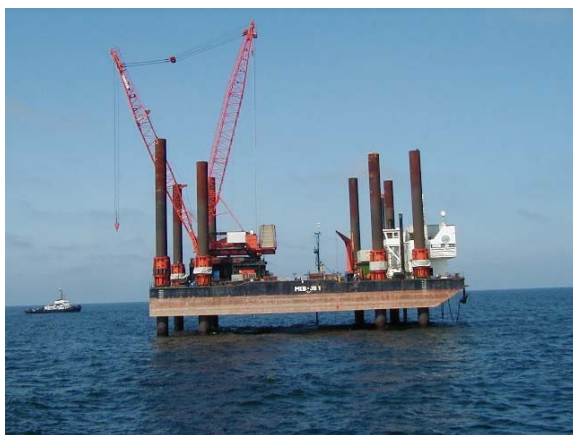
Figure 5-4: Drilling and conic penetration test with a platform from Mohiba.
