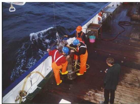
Van Veen catcher for sediment probing
