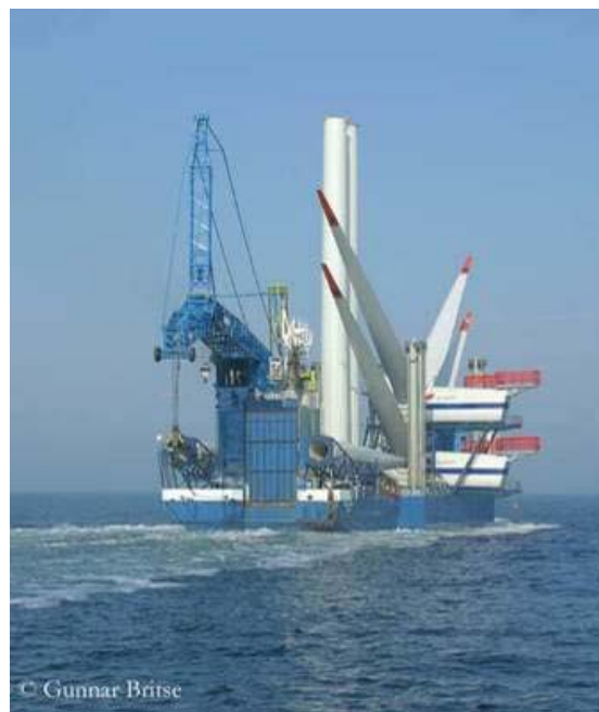
Figure 7-16: The crane vessel “Ocean Hanne” was used for turbine transport and installation (Source: Gunnar Britse).
