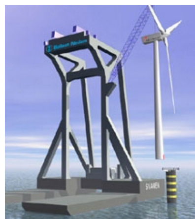
Figure 2-10: Original installation concept (source: Ballast Nedam Infra 2005).
