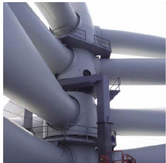
Special rack for stacking four rotors on top of each other; Source: Offshore Centre Denmark 71
