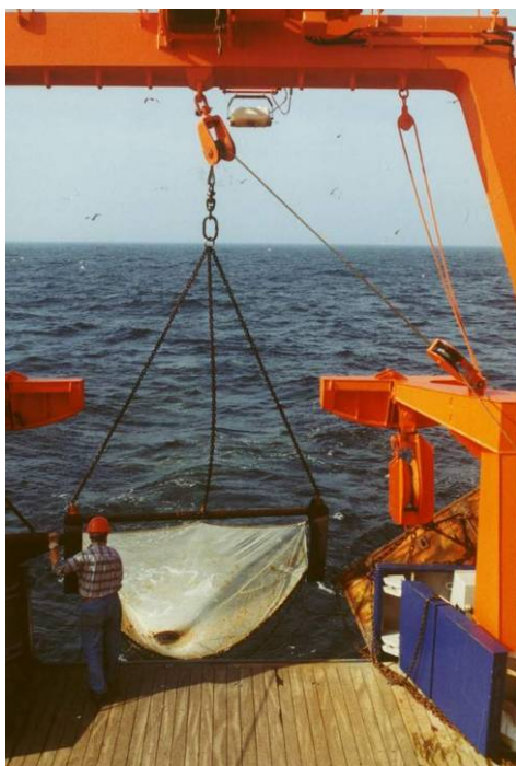
Catching fish by beam trawl
